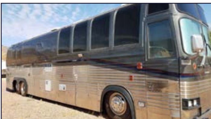
All original stainless steel was removed and replaced with a heavier gauge stainless.
