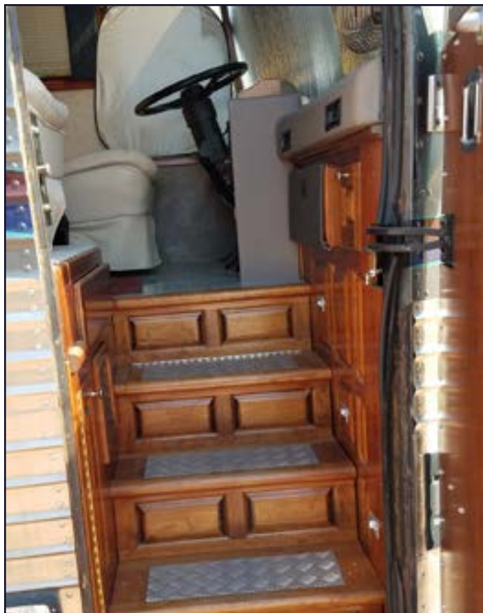
The entrance has diamond plate steps edged with cherry. Lights are along both sides of the steps.
